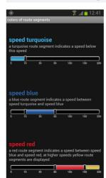
The routes displayed on the map are shown in four different colours depending on the speed.
