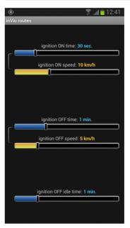
In order to display the individual sections of a long recorded route, the actual movements are recorded and displayed with an "ignition on" and an "ignition off" icon on the map. This ignition signal is sent as well to the inViu servers. In the telematic web portal inViu pro can an electronic driver log book be made using these details. More information can be found here:
