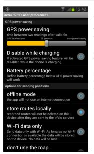
Using a slide bar the time can be set between GPS readings by GPS receiver. The greater the number, the more power is saved, but the routes recorded are only as detailed as the frequeny of the GPS readings. This power saving mode can be set depending on whether the device is charging and the battery level.
